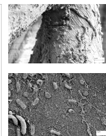
Figure 5. Bacteria attached on the surface of material removed from the capsules. (FESEM).
