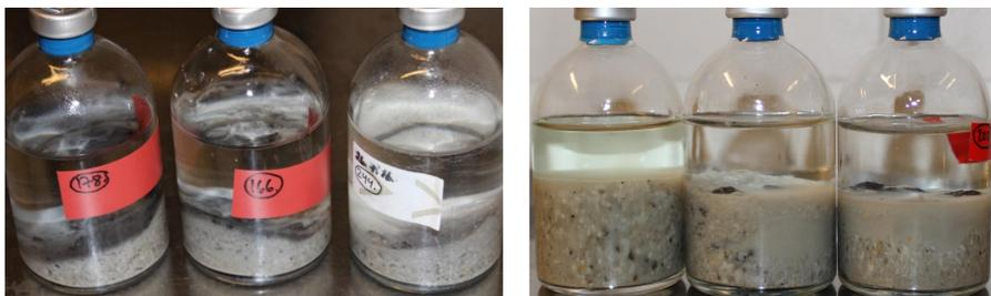
Figure 1. Sample bottles of long-term bentonite storage experiment. On the left anaerobic and on the right aerobic 120 ml headspace bottles.
