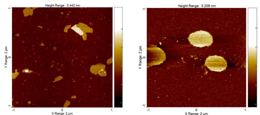
Figure 2. Atomic force microscopy (AFM) image of one month old bentonite. On the left bentonite single layers visible, on the right possible microbes (dried).
