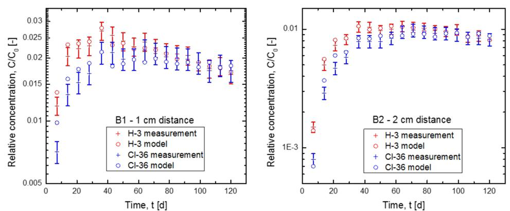
Fig 3. Measured and modelled breakthrough curves for H-3 (red) and Cl-36 (blue) to observation holes B1 (left) and B2 (right).
