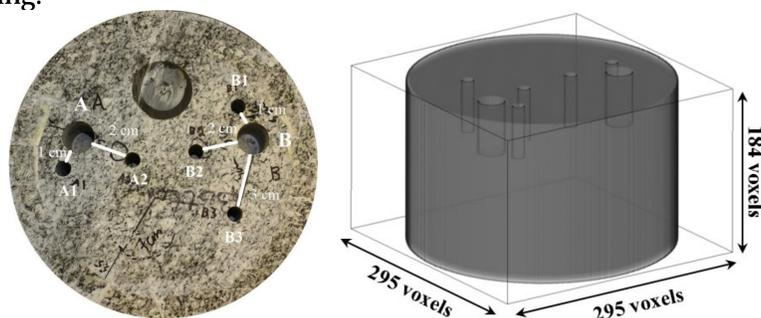
Fig. 2. Grimsel granodiorite rock block used in- and through diffusion experiment (left) and schematic drawing of experimental setup used in simulations (right).
