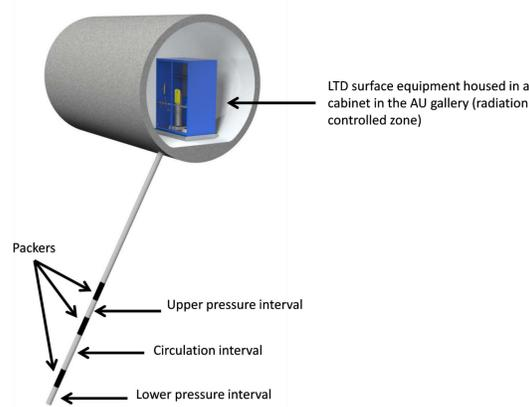
Fig. 1. Schematic illustration of the LTD in situ experiment consisting of an 8 m borehole
