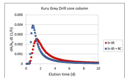
Fig. 7. The elution of Sr-85 through KGG Drill core column in the absence (red) and presence (blue) of MX-80 bentonite colloids. Allard water flow rate was 10  $\mu\text{L}/\text{min}$ .
