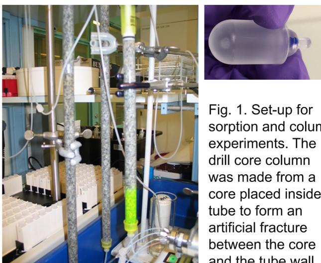
Fig. 1. Set-up for sorption and column experiments. The drill core column was made from a core placed inside a tube to form an artificial fracture between the core and the tube wall.
