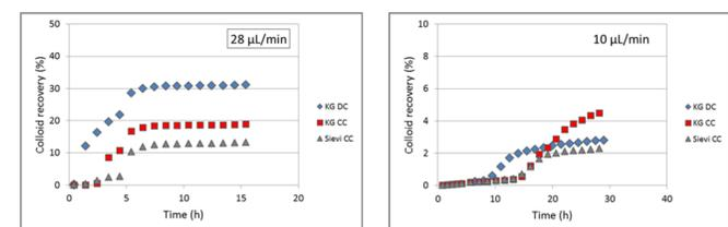
Fig. 6. Colloid recovery in KGG Drill core column (blue), KGG (red) and Sievi (grey) Crushed rock columns (15 cm). Average particle size 230 nm.
