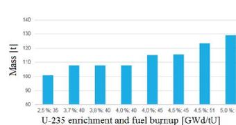
Figure 3. Total mass of plutonium and minor actinides after 100 years in 3 EPR reactors (open fuel cycle).
