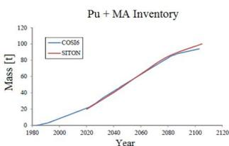
Figure 1. Total mass of plutonium and minor actinides during the simulation.
