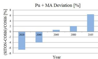
Figure 2. The difference in % between the total mass of plutonium and minor actinides calculated by COSI6 and SITON.
