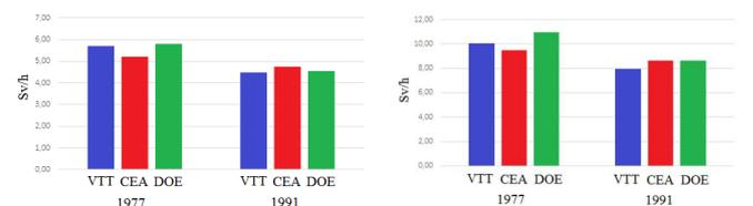
Figure 5. Gamma dose rate from UOX (left) and MOX (right) assemblies after 30 years of cooling. The numbers 1977 and 1991 refer to ANSI conversion factors used to convert the photon flux into dose rate.
