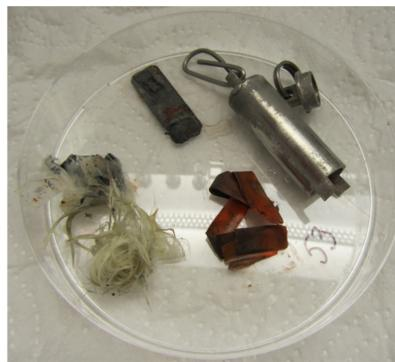
Figure 2. Capsules containing maintenance waste LLW and a piece of drum steel have been loaded to the GGE tank in 2001 and removed at certain time points (2013, 2015 and 2017) to study the corrosion rate of steel. In addition, microbial biofilms formed on the surface of waste materials and the steel plates were studied.
