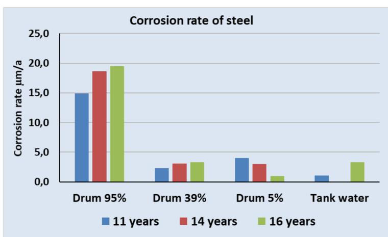
Figure 3. Corrosion rate of steel in different compartments of GGE (tank water and drums containing various amounts of cellulose) after 11, 14 and 16 years. The pH conditions inside the drums were close to neutral during the measuring period.
