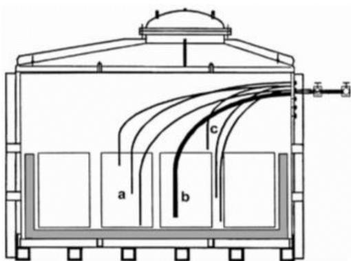
Figure 1. The GGE with waste drums containing LLW and sampling lines for water samples and capsules. The amount of cellulose-based materials inside the drums varied from 5 to 95 w-%. Before closing the GGE was filled with local river water and has been maintained at temperature of 8-11°C. (Small et al., 2017).
