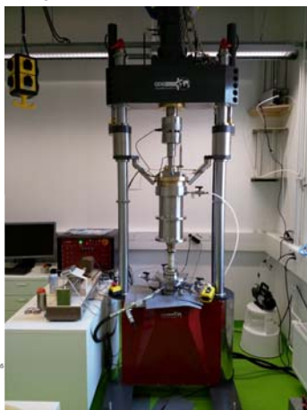
Figure 2. Loadframe + triaxial cell with sample.
