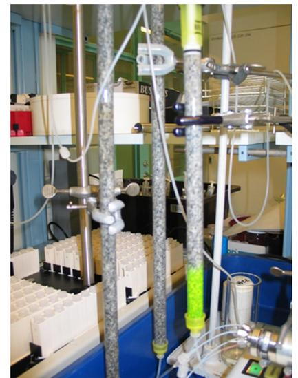
Figure 3. Experimental set-up for the column experiments.
