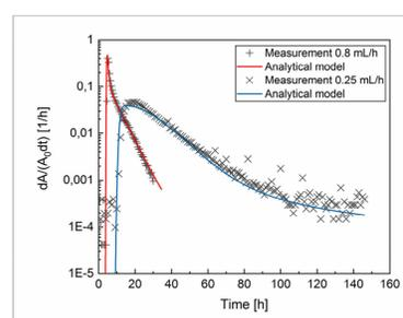
Figure 4. Measured and modeled breakthrough curves of chloride in the absence of colloids through the drill core column.
