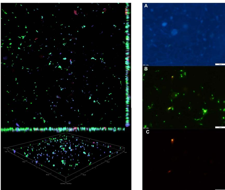
**Figure 2.** Microbes on surface of stainless steel. Blue - DAPI stained cells (non specific), Green - bacteria specific fluorescent probes, Red - Archaea specific fluorescent probes. Left panel, 3 dimensional confocal microscopy view of stainless steel surface, right panel epifluorescent views of A) all microbes, B) Bacteria, C) Archaea.
