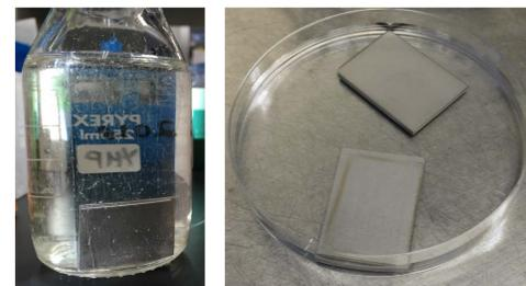
**Figure 1.** Stainless steel coupons immersed in ground water for 6 months.
